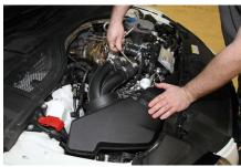
Unclip the front intake duct from the airbox, then pull up on the airbox to remove from the rubber mountings. Ensure you leave all three of the rubber mountings in place as they will be reused.
